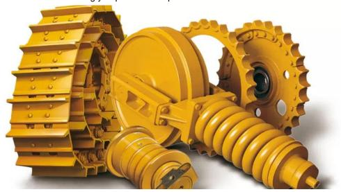
Excavator carrier roller is made of shell, bronze bushing, collar, seal, lock pin, plug, shaft. It is made by forging, machining, heat treatment, assembly, painting etc. The quality and working life for excavator carrier roller is depends on the quality of raw steels, the hardness of rail surface, the depth of hardness layer, the quality of seal group etc.
