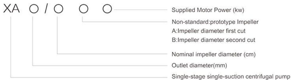
E.g. XA32/13A means pump outlet diameter is 32mm, the impeller nominal diameter is 13cm. Impeller is after the first cutting.
