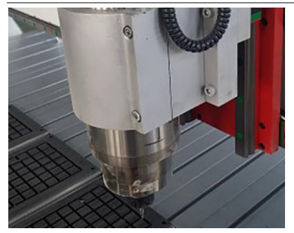
• High Speed 5.5KW Water Spindle
