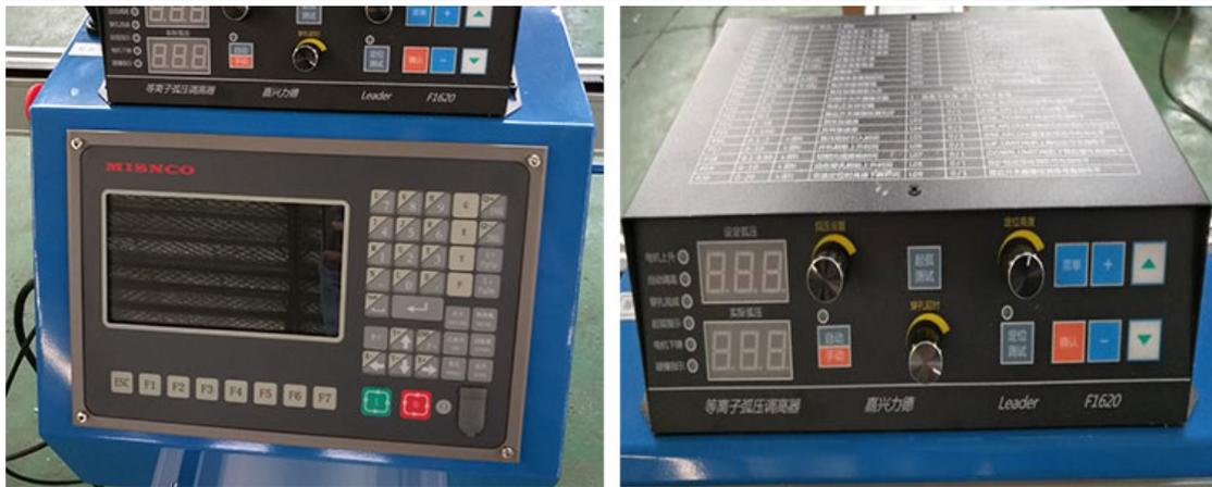
A cut drawing library with rich resources is built into the cnc system. Production cuts can be executed by simply setting the size parameters.
