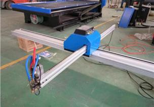
The default configuration coming with two torches, one plasma cut torch, and one Oxyfuel flame cutting torch.
