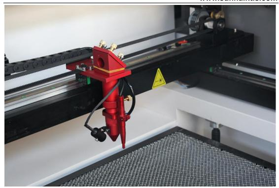
High quality laser head with red light positioning system,imported lens which will make the light beam stable and powerful. Air-cooled system to protect the lens and laser head.
