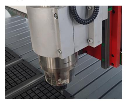
• High Speed 5.5KW Water Spindle
