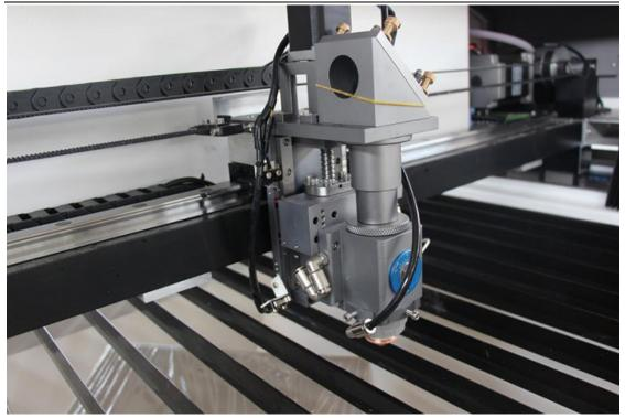
Mechanical follow-up cutting head system, cutting head always follows the material to keep the cutting point location unchanged, which insures smooth cutting section without processing again.
