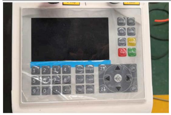
RD control system: there has the USB interface in the control panel, do not need to connect into the computer, supporting offline work, very convenient.
