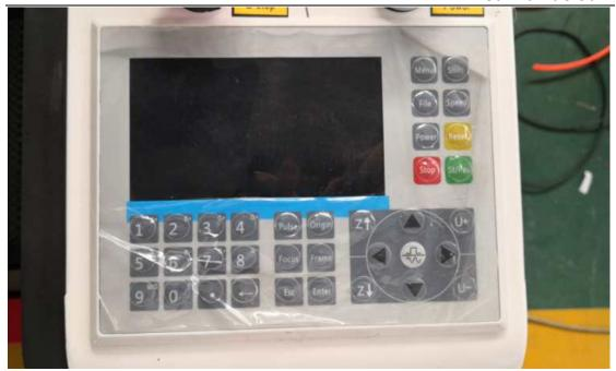
RD control system:there has the USB interface in the control panel, do not need to connect into the computer, supporting offline work, very convenient.
