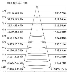
Height Eavg, Emax Angle: 55.63 deg Diameter Note: The Curves indicate the illuminated area and the average illumination when the luminaire is at different distances.
