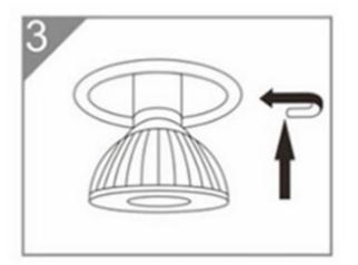
3.Insert and turn the GU10 MR16 in the fixture or lamp stand and make sure it is fixed.
