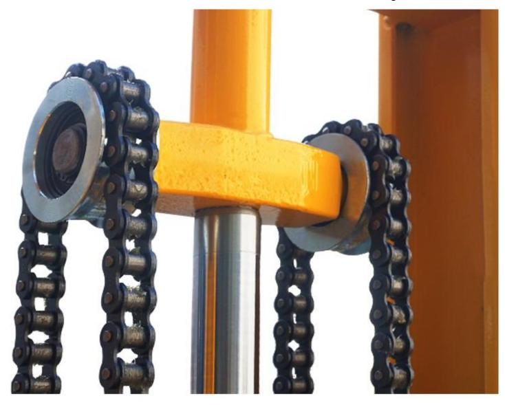
③Manual Pallet Lifter has labor-saving durable oil cylinder.Convenient operation and labor saving.
