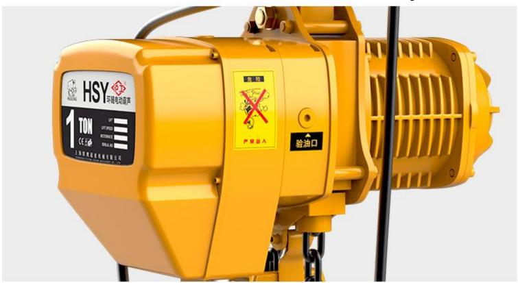
The electric hoist 1 Ton is equipped with a limit switch, which automatically stops when the goods are pulled to the top to prevent impact on the hoist and damage to the hoist. It stops automatically when it is at the bottom to prevent the chain from exceeding.
