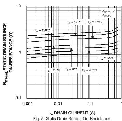
Fig. 5 Static Drain-Source On-Resistance
