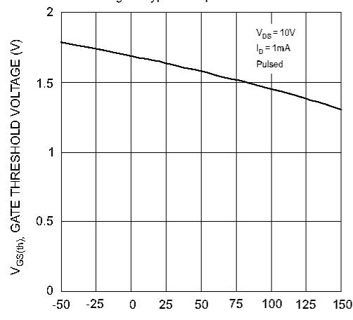
Fig. 3 Gate Threshold Voltage
