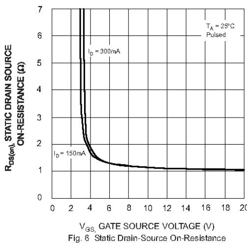
Fig. 6 Static Drain-Source On-Resistance
