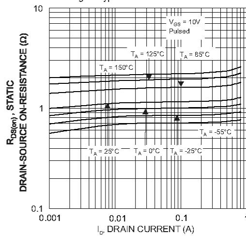
Fig. 4 Static Drain-Source On-Resistance
