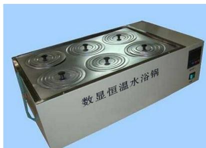
Timed constant temperature porous water bath is widely used for drying, deep shrinking, vegetable distillation, impregnating chemical reagents, impregnating pharmaceutical drugs and biological products, and can also be used for constant temperature heating in water bath and other temperature tests. It is biological, genetic, virus, aquatic, environmental protection, medicine, and health. , Biochemical laboratory, analysis room, essential tools for education and scientific research.
