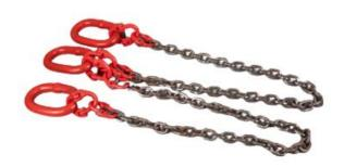
The chain of this Chain Slings with G80 Master Link is made of G80 Mn-steel, the hoist links and hooks are powder coated alloy steel, which is wear resistant and resistant to high temperature welding. Chain Sling is a convenient lifting tool made of lifting ring and double leg sling chain with grab hook. The chain of this sling chain uses fully automatic welding and is designed for long-term use.
