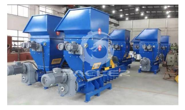
Packer Machinery is just making the EPS compactor to solve this problem, it can reduce the size of the EPS material, the compressing ratio can reach 1:30-1:50. The finished products is the EPS blocks, the density can reach 350kg/ m3. It is easy for the customer to deliver the EPS material to another recycling processing unit.
