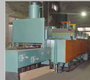
▲ Belt Heat Treatment Furnace 热处理炉
