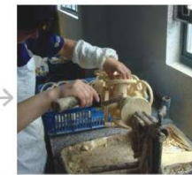
▲ Wax Model Assembly 蜡树组树
