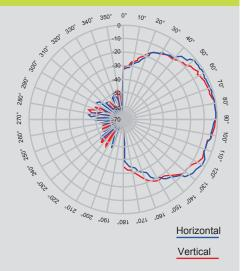
PD-V6 5.8GHz 180°Microwave Motion Sensor is a C-Band Bi-Static Doppler transceiver modlue .It's built-in Resonator Oscillator (CRO).This module, which uses the built-in amplifier circuit and directly outputs amplification signal, V6 adopts flat Plane Antenna, suitable for wall mounting. It can improve its front signal receiving ability and reduce its flank blind area. Its performance is better than the sensors in the market.
