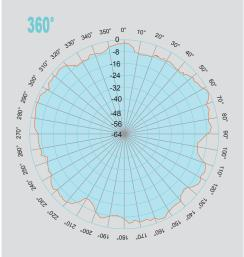
PD-V5 360° 5.8GHz Microwave Motion Sensor is a C-Band Bi-Static Doppler transceiver modlue .It adopts built-in Resonator Oscillator (CRO) amplificated signal external circuit.More sensitive and lower power consumption than V2 $_{\circ}$  It is convenient for the customers to develop various products.
