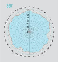
PD-V3 360° 5.8GHz Microwave Motion Sensor is a C-Band Bi-Static Doppler transceiver modlue .It adopts built-in Resonator Oscillator (CRO) amplificated signal external circuit.More sensitive and lower power consumption than V2. It is convenient for the customers to develop various products.
