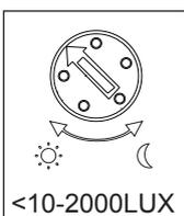
Adjust working light. Turn clockwise to increase it and turn anti-clockwise to decrease it. When turn to mini, it will only work below the light-control about 10LUX, when turn to max, it can work any light-control.
