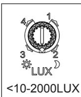
The work illumination value can be adjusted <10-2000LUX range.
