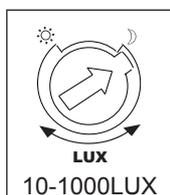
It can be defined in the range of 10~1000 LUX. To turn fully anti-clockwise is about 10 lux, fully clockwise is about 1000 lux. You are supposed to turn fully clockwise during the daytime walking test or adjustment of detection range, in this case, the LED lamp controlled will keep on however the ambient light is.
