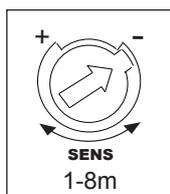
Detection range is the term used to describe the radii of the roughly circle casting on the ground when installed at the height of 2.5 m. To turn fully anti-clockwise is the minimum distance (approx. 1m), fully clockwise is the maximum (approx. 8m). If person's stature, figure and moving speed change, the detection will also change, that is, the higher speed will lead to the shorter detection distance.
