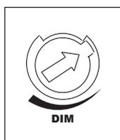
It can be defined in the range of 0%~10%. When the ambient light is less than 70 lux, the system starts dimming mode. If there is no signal detected during the delay time, it will enter the percentage lighting. Once signal detected, it recovers to 100% lighting. It will auto exit dimming mode, when the ambient light is over 100 lux. The dimming mode works digitally and independently.
