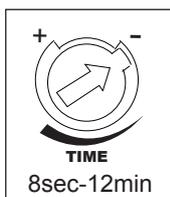
When motion signal detected, the LED lamp controlled be auto on. And if there is no signal during the delay time (8s ~12min), it be auto off and you're expected to wait for 4 seconds before the next detection. And any motion signal detected during the customer-defined time will lead the system re-compute the time. It is suggested you choose the minimum time during test to save energy & time.
