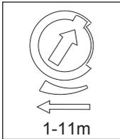
Detection range is the term used to describe the radii of the roughly circle casting on the ground when installed at the height of 2.5 m. To turn the knob fully anti-clockwise is the minimum range, fully clockwise is the maximum.
