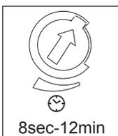
It can be defined from 8 seconds (turn fully anti-clockwise) to 12 minutes (turn fully clockwise). Any movement detected before this time elapses will re-start the timer. It is recommended to select the shortest time for adjusting the detection range and for performing the walk test.
