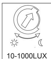
It can be defined in the range of 10~1000 LUX. To turn the knob fully anti-clockwise is about 10 lux,fully clockwise is about 1000 lux.When adjusting the detection zone and performing the walk test in daylight,you should turn the knob fully clockwise.
