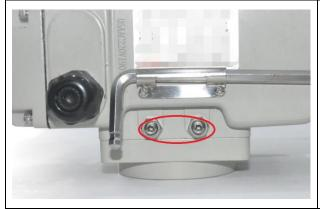
Ordinary nuts are used for the mechanical limit part, which will easily fall off due to field vibration, resulting in over travel or locked rotor, resulting in inaccurate positioning.
