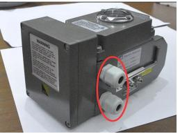
The valve actuator produced by other factories only uses one terminal when it is manufactured. All power lines and signal lines are connected to
