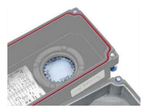
Using the "AOX-R" series motor operated valve actuator, we can observe through our lens structure. The lens structure is a mechanical sealing structure, not a chemical adhesive used by other factories, to avoid the insufficient sealing of the brake due to the aging of the chemical adhesive under high temperature and high pressure.
