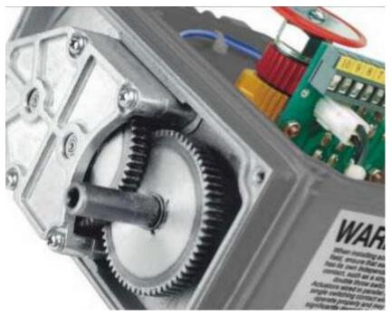
2. AOX makes the motor temperature rise lower by increasing the size of the motor. The principle is that the capacitor capacity is reduced for the same power, lowering the starting current and reducing the degree of heat generation.
