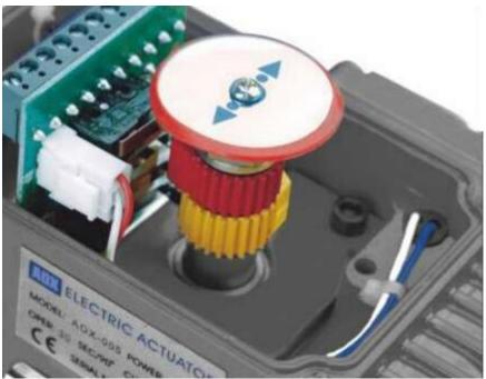
The appearance of AOX-R series electric part turn butterfly valve actuator has been upgraded for several times, and now its appearance is very novel and beautiful. The shell adopts high-strength die-casting aluminum shell and anti-corrosion coating, which improves the internal sealing condition of the electric actuator and improves the service life of the valve actuator.
