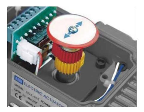
3. More convenient and reliable assembly with the valve: the same way of coupling with the pneumatic actuator, more conducive to the unification of standards, can effectively reduce the valve inventory. And the valve stem is directly inserted into the internal worm gear of the actuator, which makes the force arm of the valve and the force shaft shorter and the force more stable.
