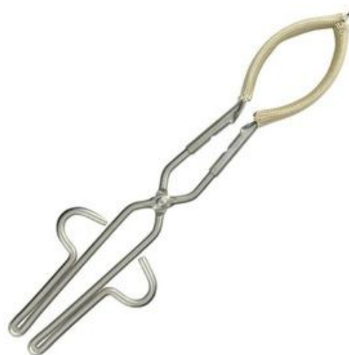
HSG-212 Stainless Steel Beaker Safety Tongs with Fiberglass Covered Jaws for 100mL to 1,500mL Beakers, 13.5" Length
