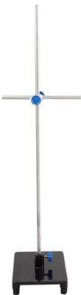
HSG-072 Physical Lab Cast Iron Universal support Stand with the clamp and rods
