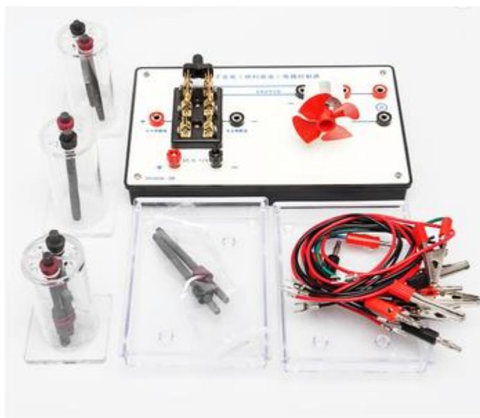
HSPEN-032 Hydrogen gas system electricity generator
