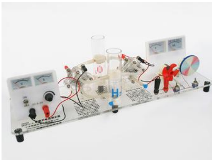
HSPEN-009 Hydrogen fuel cell demonstration
