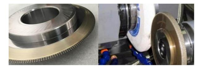
The basic principle is to change the original single point of the original diamond dresser into rotary dresser trimming, which is divided into swing type and fixed type according to the dressing tool dressing method. Most of the common ones are fixed, and they are moved and trimmed according to a certain trajectory to repair the partial surface.
