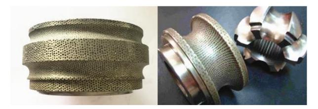
Here selected diamonds are applied to the negative profile by hand using an adhesive and in accordance with a defined pattern. By varying the distances between the diamond grits, it is possible to achieve the optimum arrangement of diamonds needed to ensure the required surface finish later in the workpiece.
