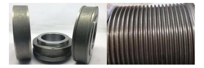
The diamond grit size, selected to correspond to the smallest convex profile radius, subsequently determines the surface finish of the workpiece to be ground so that small radii and relative coarse surface qualities do not correlate. Here the diamonds are packed next to each other as densely as possible in a stochastic distribution. This is beneficial for the tool life of the roll but also leads to increased dressing forces.
