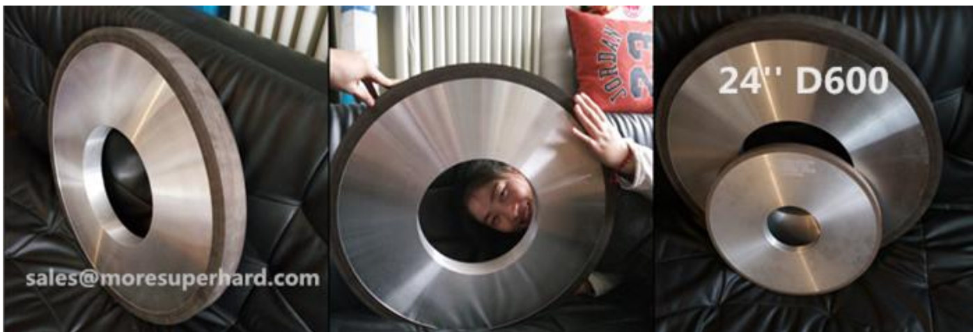
24 inch ( D600mm) Resin bond diamond grinding wheel
