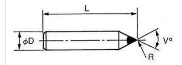
Application: dressing specific forms into conventional abrasive wheels(formingarc, angle, groove radius and other complex profiles).
