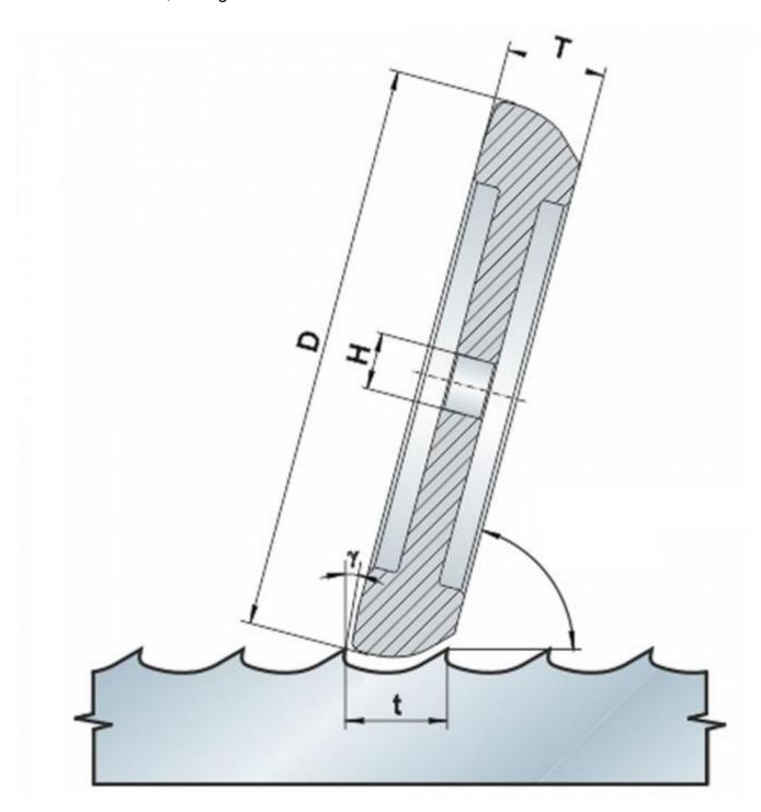
Main Features of CBN grinding wheel for band saw blade sharpening
