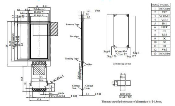
**Product Interface Pin Function of the 0.96 inch OLED Display**
