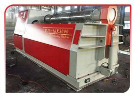
Full hydraulic 4 roll plate bending machine is a machine which 4 rollers rotate and move are controlled by hydraulic, this kind of bending machine is mainly used for large workpiece.
