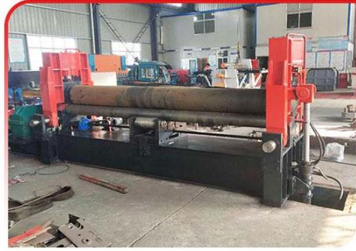
The hydraulic 3 roll plate bending machine is used for rolling the plate into cylindrical shape, circular arc shape and conical shape under normal temperature. The machine with below features
