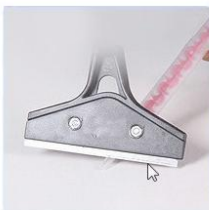
2. Cut the nozzel according to the width of the gap
