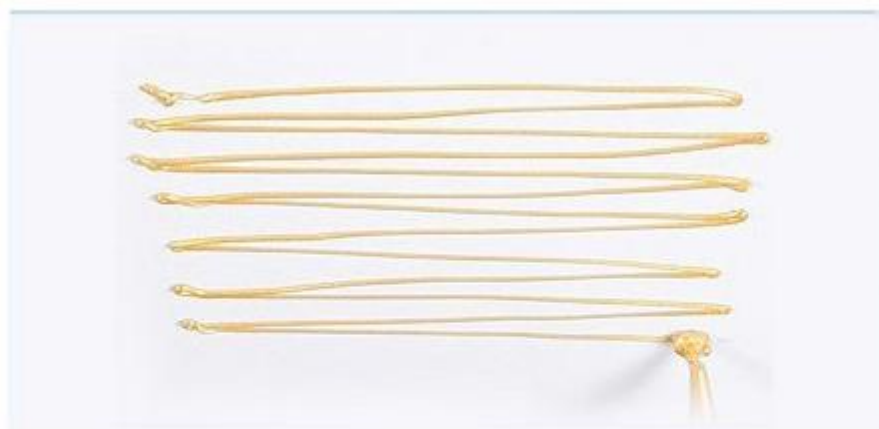
4. Before application, first 30-40cm has to waste because it is not fully mixed.
