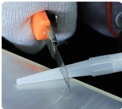
4.Cut Nozzle To Desired Based Size
