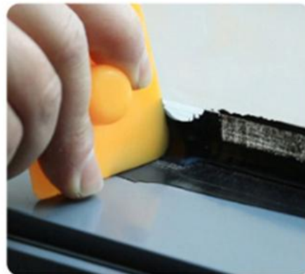
8.Scrape off Any Excess Glue
